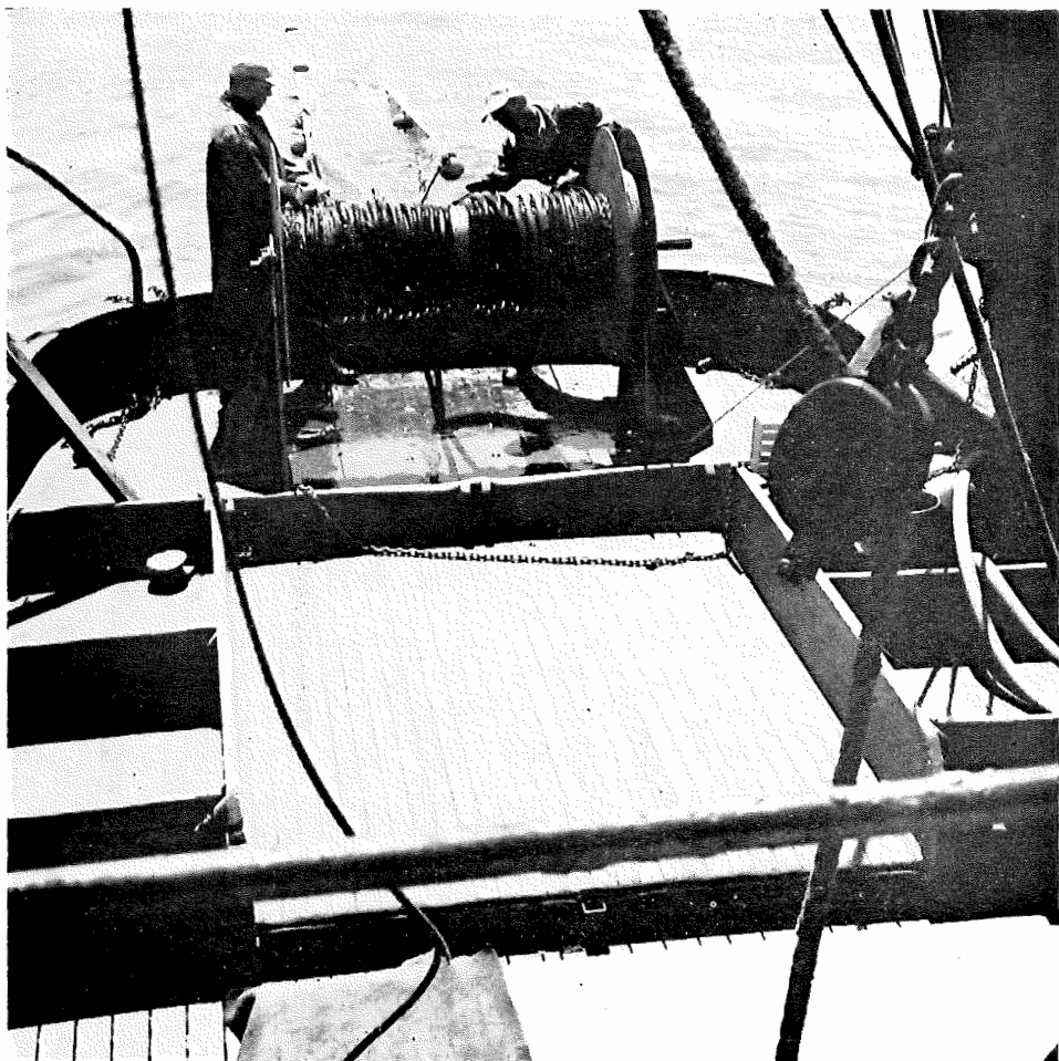
FIGURE 7. REEL ON THE STERN OF THE MARIAN F. SHOWING THE CABLES BEING WOUND IN, WITH THE NET IN THE WATER IN THE BACKGROUND.
