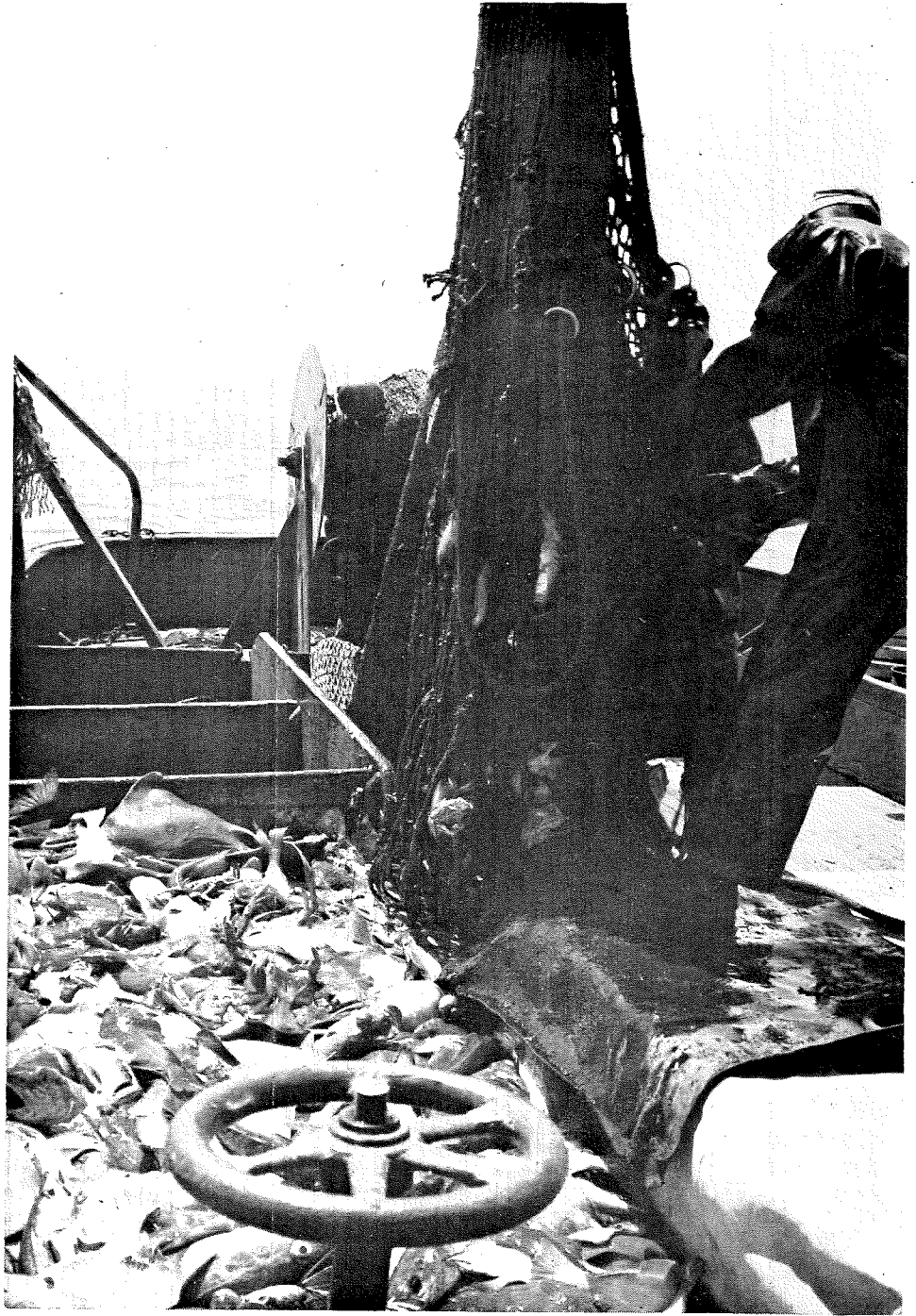
FIGURE 8. SHOWING THE COD-END HOISTED AND SPILLED AFTER THE REMAINDER OF THE NET HAD BEEN WOUND ON THE REEL ON BOARD THE MARIAN F.
