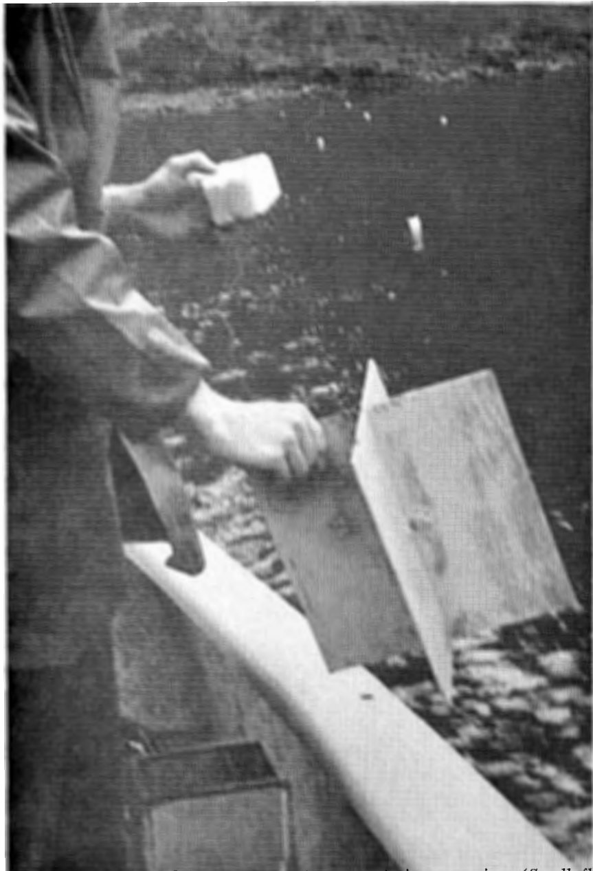
Figure 2—The drogue used to measure water currents in reservoirs. (Small floats supporting vanes of other drogues are visible in background.)
