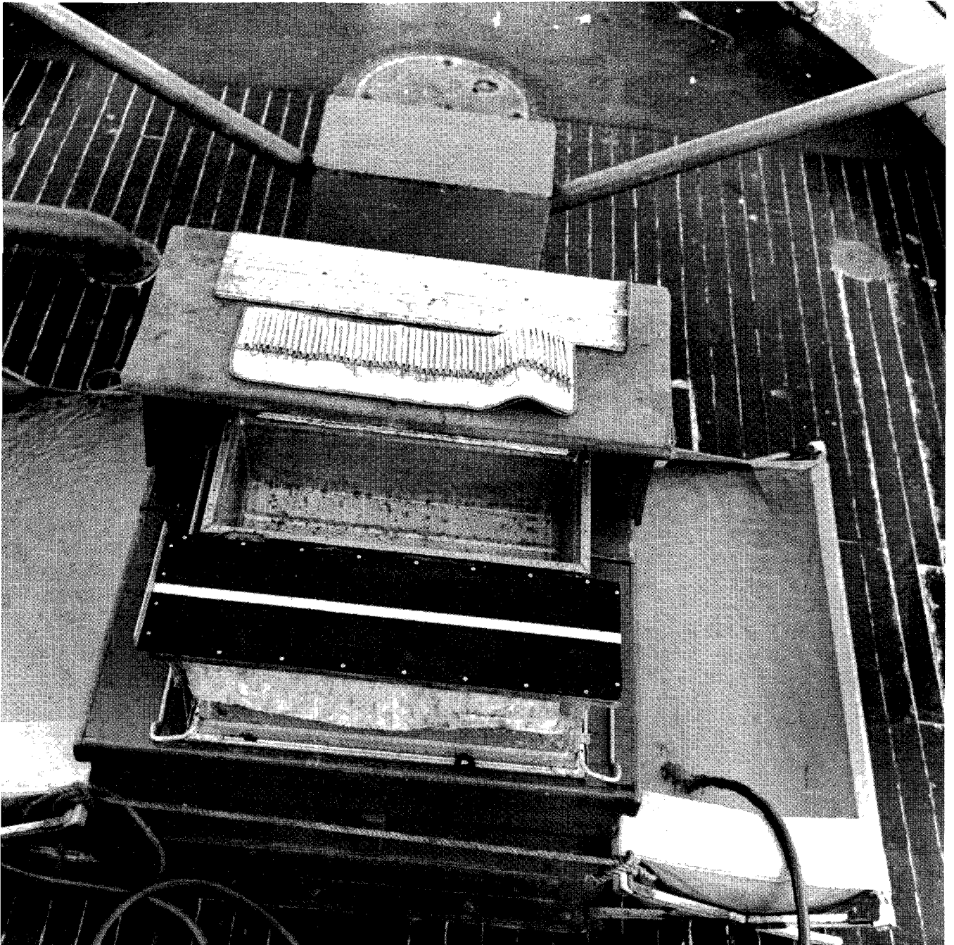
FIGURE 1. Facilities for tagging aboard the N. B. Scofield . Live tanks, measuring boards and spaghetti tags ready for use. Photograph by author, December, 1960.
