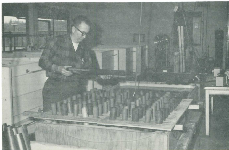
Figure 2. Larval rearing tank with polyvinyl pipe being tested as cultch material
