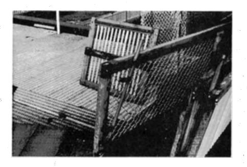
This crowder at Big Creek Hatchery has a handle to lock it in place when in use. Top photo shows handle in unlock position and bottom in locked position.
