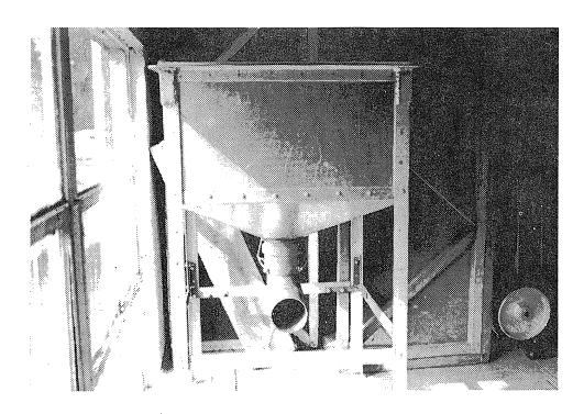
This fish distribution unit can be placed on a pickup truck or battery-powered cart and is currently being used at Marion Forks Hatchery.
