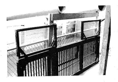
Clackamas Hatchery uses this crowder. It has an upper section that can be folded down as shown above allowing employee to easily crawl over or be raised as shown below while crowding fish, this preventing fish from jumping over.
