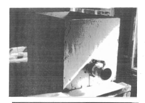
The upper and middle photos show the fish distribution box plumbed with plastic pipe and is in use at Salmon River Hatchery. The box below is designed for irrigation pipe and is in use at Alsea Hatchery.
