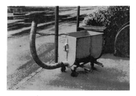
This unit can either be rolled by hand or moved around with a forklift to accommodate fish distribution within the hatchery. This unit is located at Gnat Creek Hatchery.
