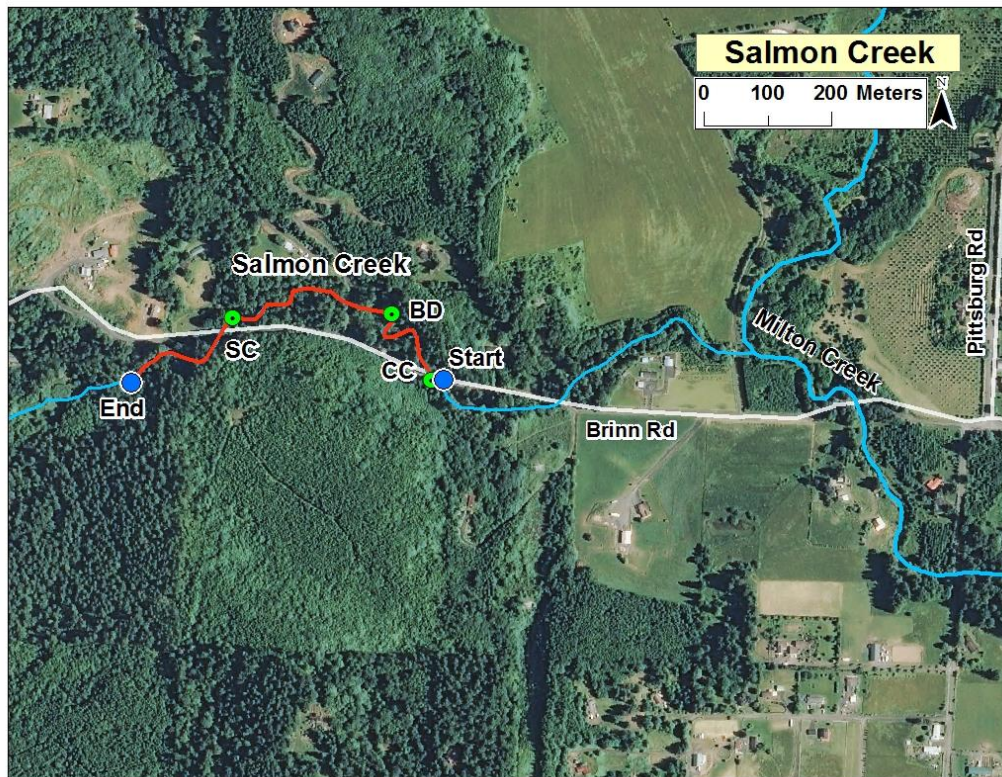
Figure 44. Map of reach (red line) surveyed on Salmon Creek, located west of St. Helens, OR, including start and end points (blue dots), a circular culvert (CC), a beaver dam (BD), and a semicircular culvert (SC).
