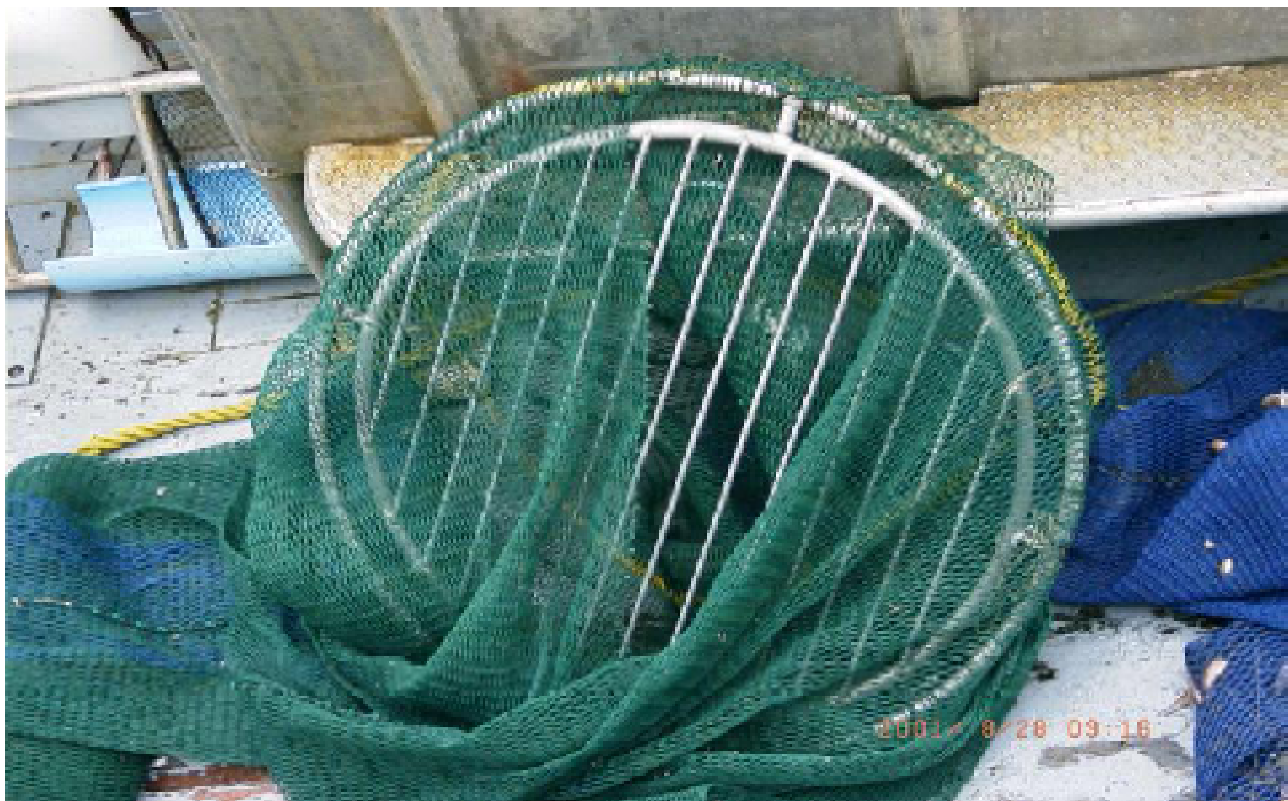
Figure 3. A photograph of one version of the Nordmore grate that was developed by Jeff Boardman and used successfully on the F/V Miss Yvonne during 2001.
