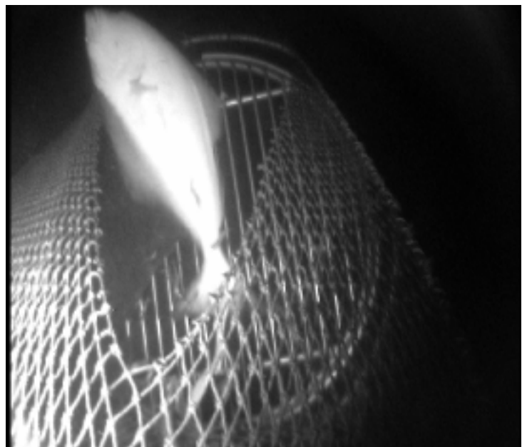
Figure 4. A Pacific halibut being excluded from a round grate BRD. The camera was mounted ahead of the BRD aperture looking aft. The footage was taken while shrimping in 2003 aboard the F.V. Miss Yvonne.
