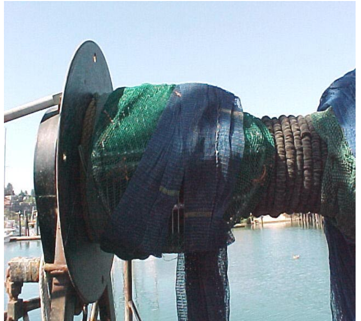
Photo 4. A shrimp net and folding Oregon Grate being reeled onto a double-rig Oregon shrimp vessel. The intermediate, body and footrope gear can be guided toward the center of the reel to relieve stress on the grate. Here again, stout construction can help reduce grate distortion. Also, a BRD may be loosely, but securely, tied into the net on the sides to reduce pull on the web as the BRD folds. However, any slack created between the net and grate must not allow a 110 mm (5.5") ball to pass through in any configuration.
