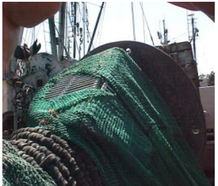
Photo 5. A second view of a folding Oregon Grate as it's reeled onto the stern reel of a double-rig Oregon shrimp vessel.
