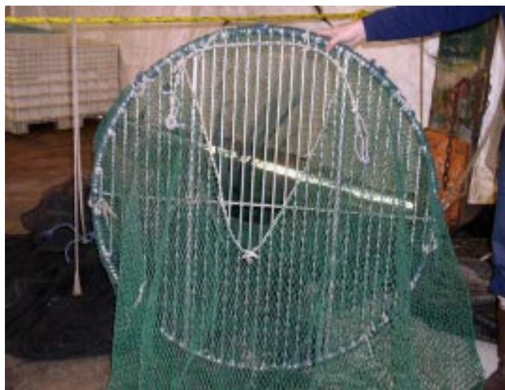
Photo 1. A single-ring Oregon Grate (1.25" bar spacing) mounted in a net of a double-rig Oregon shrimp vessel.
