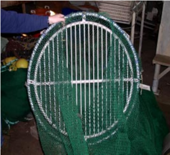
Photo 2. A double-ring Oregon Grate (1.25" bar spacing) with a removable grate panel used on an Oregon double-rig shrimp vessel. The removable panel makes it possible to switch to a panel with a different bar spacing without removing the entire BRD. Shrimpers report mixed opinions about whether a double-ring is necessary.
