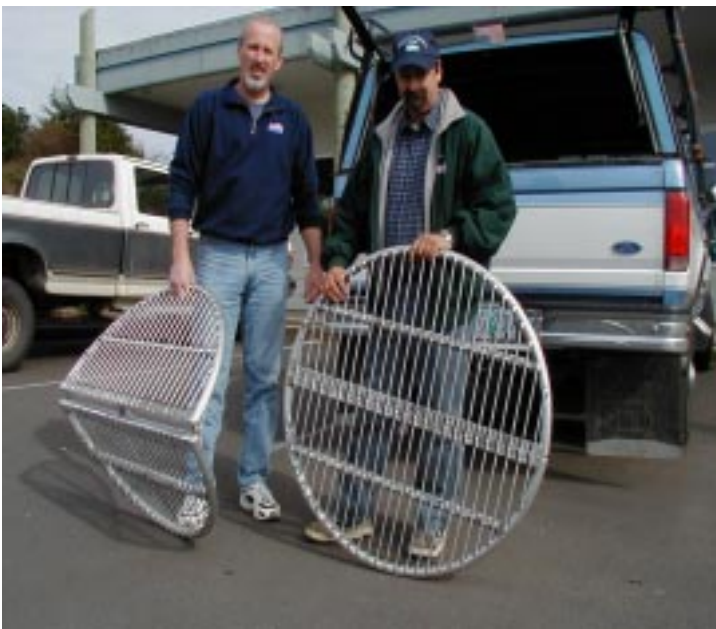
Photo 3. Mr. Brad Pettinger (F.V. Alex) and Mr. Gerald Gunnari (F.V. Coast Pride) holding stoutly built hinged aluminum grates (1.25" bar spacing). The grates are designed for rolling onto the stern reel of double- or single-rig shrimp vessels. The heavy construction helps reduce bending of the BRD when the net is reeled on top of it. A folding grate can be constructed to fold either forward or backward, depending on how a vessel reels it's net(s) aboard.
