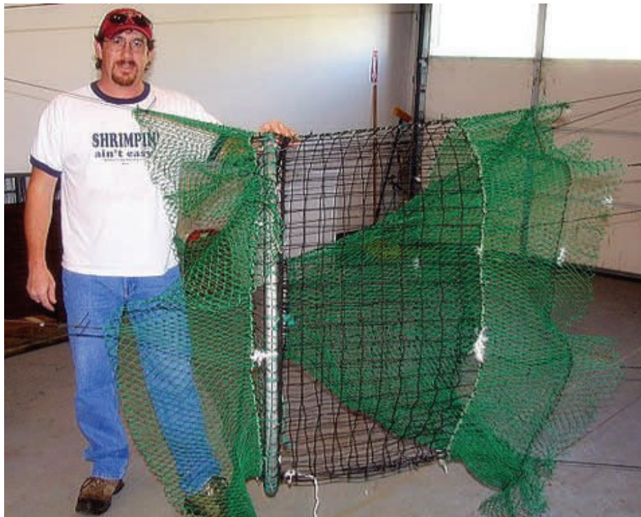
Figure 19. Corey Rock, who fishes the F.V. Kylie Lynn, stands at the aft end of the "expanded mesh" BRD he designed to help exclude "mini" hake that passed through his rigid-grate BRD. The device was installed between the rigid-grate (not shown, but to the right) and the codend (not shown, but to the left). Shrimp and small fish pass through the rigid-grate and are funneled back into the codend. In theory, fish can swim forward and out the expanded meshes after entering the codend.
