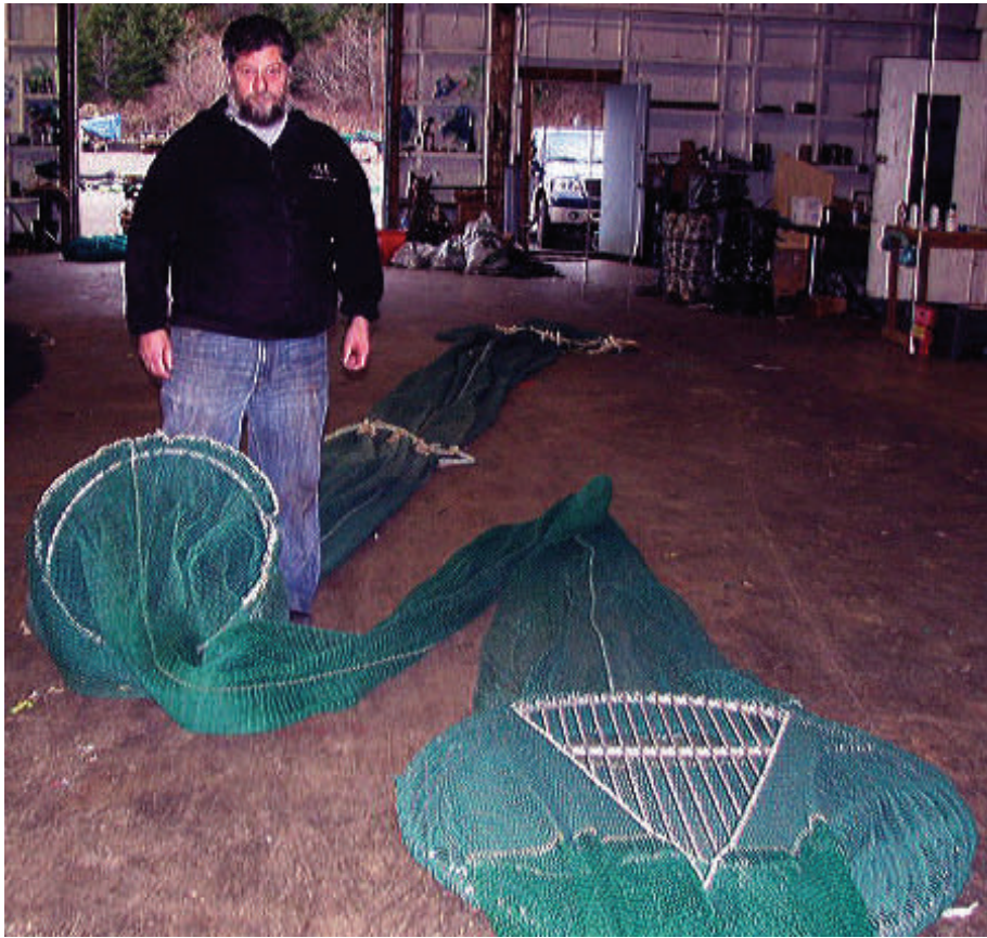
Figure 20. John McMillan, who fishes the F.V. Evolution, showing his “accelerator ring” setup. The ring, shown braced against John’s knee, is laced in at the forward end of the codend behind his rigid-grate BRD.
