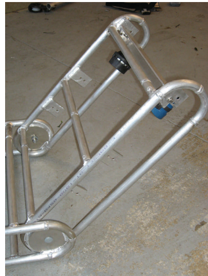
Figure 19. The forward end of the "Hayladder" with the camera and light attached. Imagine the fishing-line passing below and slightly behind the circular hinge plates. Look for more photos of the device in place in next years' Review!
