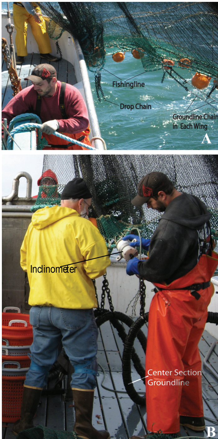
Figure 20A & 20B. Views showing a shrimp trawl we used in our groundgear experiment last summer. The top photo shows the trawl with the center section of groundline removed, with just droppers remaining. The bottom photo shows the “doughnut” covered center section in place. A recording inclinometer is shown in the lower photo.
