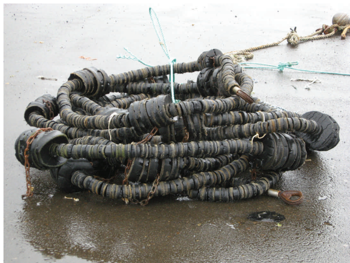
Figure 18. A detached "heavy" groundline. Note that the groundline is covered continuously with rubber "doughnuts" (3" & 8" diameter) from wingtip to wingtip.
