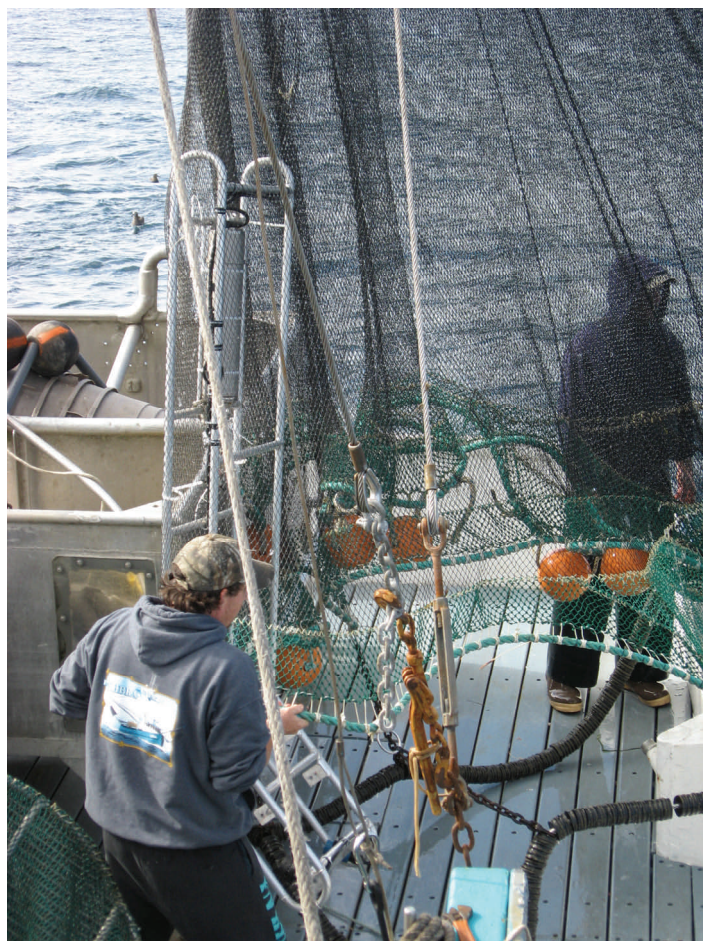
Figure 19. The "Hayladder" mounted inside the shrimp trawl, extending out in front of the fishingline. A camera and light point back for a view of the groundgear in action.
