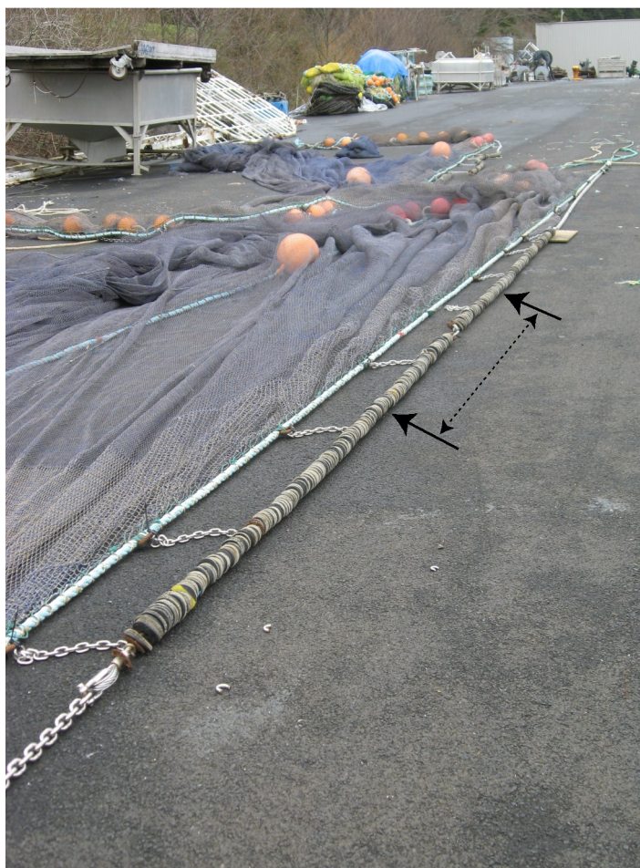
Figure 20. Photo showing one of the nets we tested during our “footrope window” experiment with a complete groundline. The dark arrows designate the groundline section that was removed on the other net
