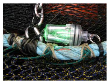
**Figure 2**. Photo of a single green Lindgren-Pitman Electralume light zip-tied to the fishing line of a shrimp trawl. We found that looser zip-ties worked better to avoid torqueing the light.
