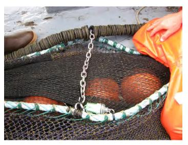
**Figure 3**. The same light shown in Figure 2 showing its relative position to the chain droppers and doughnut-covered groundline. While fishing, the fishing line was about 15 inches above the groundline on each net.
