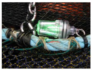
Figure 18. Photo of a single green Lindgren-Pitman Electralume light zip-tied to the fishing line of a shrimp trawl. We found that looser zip-ties worked better to avoid torqueing the light.
