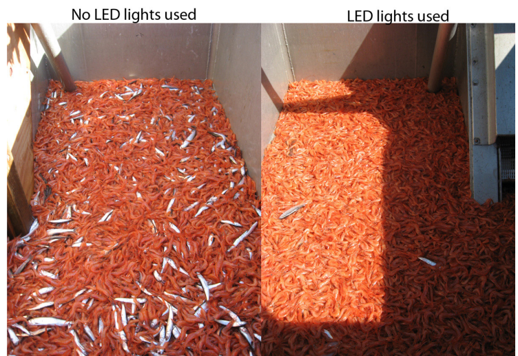
Figure 19. a divided shrimp hopper where no LEDs were used on the left side and LEDs were used on the right side, notice the marked difference in eulachon smelt (the silver fish).
