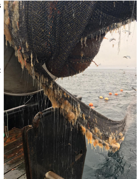
Figure 21. Jellyfish fouling a shrimp net (photo courtesy of Matt Hakki, F/V Big Wave)
