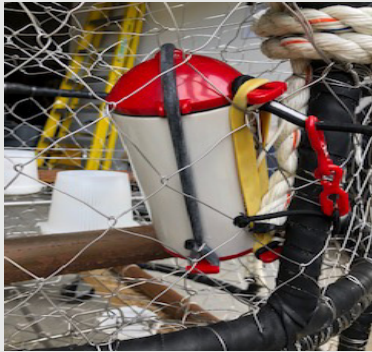
A bottom-water sampler attached to a crab pot to collect information on HAB concentrations at depth.
