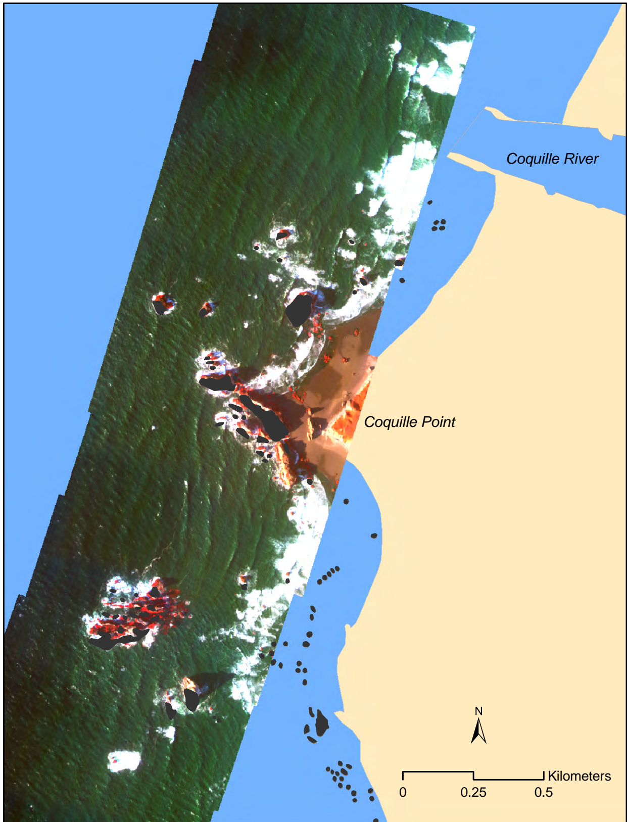
Figure 8b. Digital multispectral imagery mosaics of kelp canopy at Coquille Reef. Reflectance signatures in the near-IR part of the electromagnetic spectrum isolate live vegetation. Exposed (and some submerged) kelp show a very strong reflectance signature in the DMSC band 4. Depth penetration was estimated to be roughly one meter.
