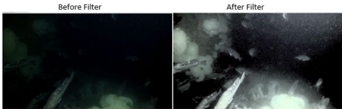
Figure 7. Example of applying a filter to increase ability to identify fish to species and/or take accurate length measurements
