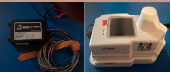
Picture: The two vessel monitoring systems, Faria Beede Sentry 350 and Woodhole NEMO, that will be tested throughout the crab electronic pilot project. Photos courtesy of Harbor Lights Software.
