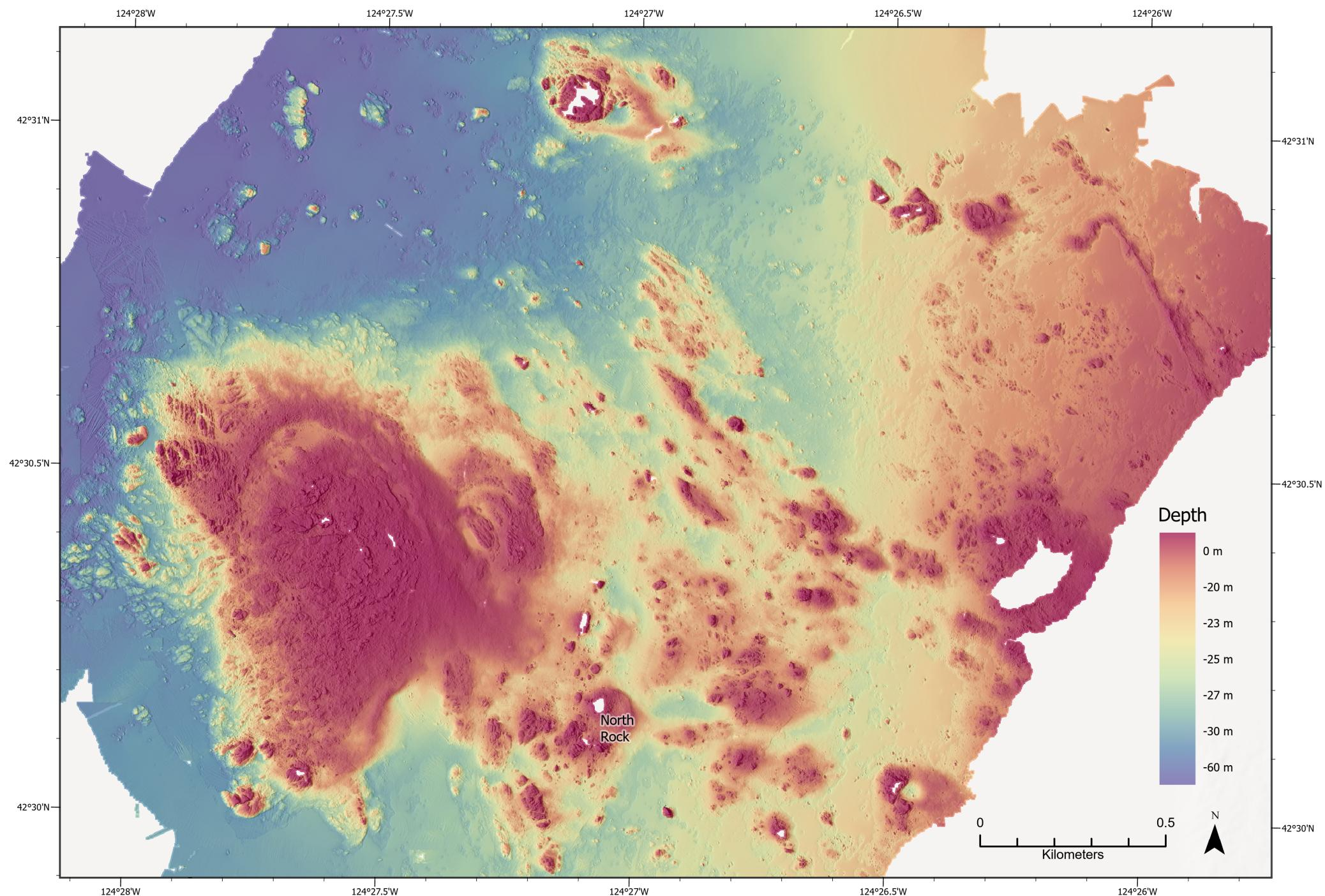
Detail view of ODFW bathymetry survey data at Breakers Reef. Areas in white are data gaps, and may represent features that presented hazards to navigation during the survey (islands, submerged rocks, mounding waves, or kelp at the surface), or simply gaps between survey vessel transits. Map not intended for navigation.
