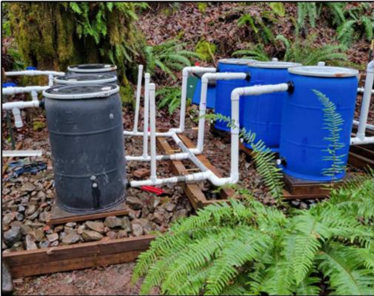
Figure 6. The remote site incubator (RSI) constructed alongside Page Creek in the Clatskanie River Recovery Population used to house Chum Salmon ( Oncorhynchus keta ) eyed-eggs in 2022–2024. Water flows into the blue filtration barrels from two intake pipes secured in Page Creek. From there, water flows into the black barrels holding the eyed-eggs, each of which has an outflow pipe to allow fry to leave volitionally.
