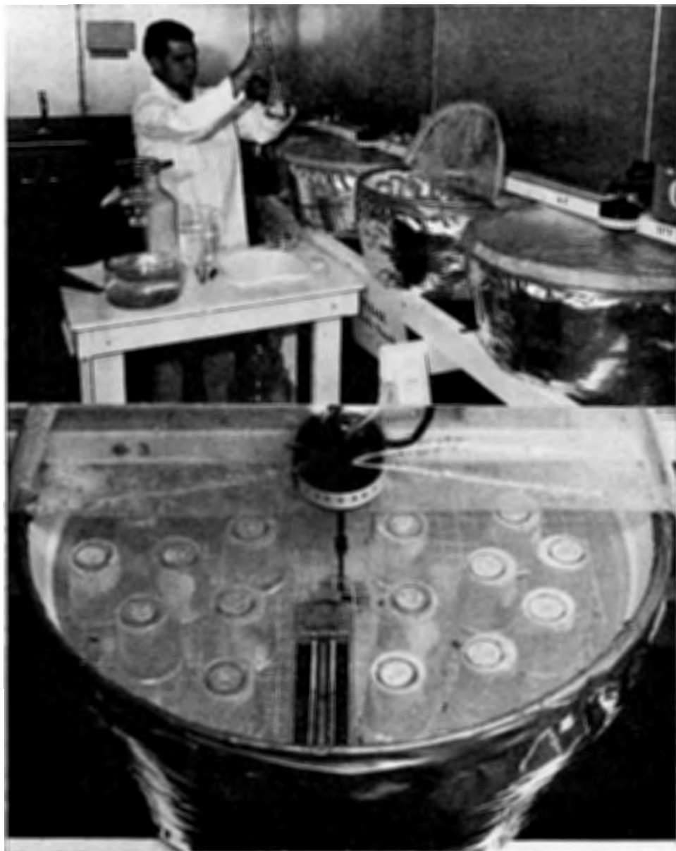
FIG. 1. Water baths in a constant temperature laboratory showing dispensing of food to a culture flask ( top ), and a detailed view of a water bath ( bottom ).
