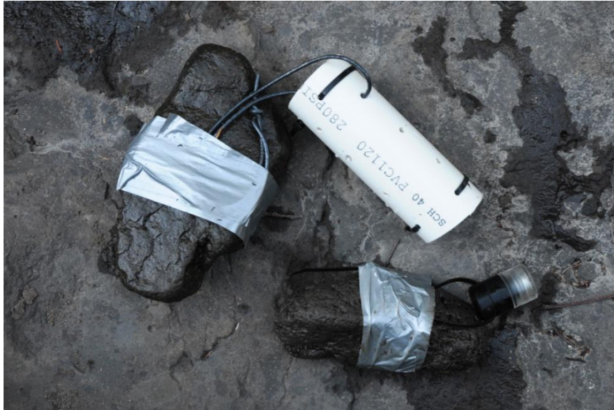
Fig. 1. A NexSens® data logger in the waterproof housing, lower right, and another in the same housing but further encased in a section of PVC pipe. This photo is from a test comparing temperatures recorded by shielded and unshielded loggers.
