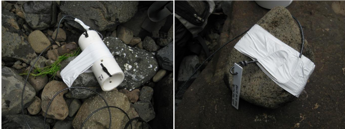
Fig. 1 (left). Data logger inside protective housing, with anchor, ready to be placed in the water. Fig. 2 (right). Cable anchoring method used when there is no convenient root wad or other structure for securing the cable. In this case, the cable anchor is placed in the water behind a boulder upstream of the anchored data logger, or at a secure spot on the bank.
