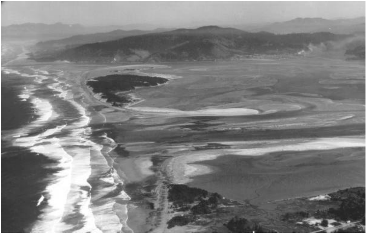
Figure 1-2. Waves carry sediment through Bayocean Spit into Tillamook Bay in this May 1954 photo, 1 1/2 years after the breach.
