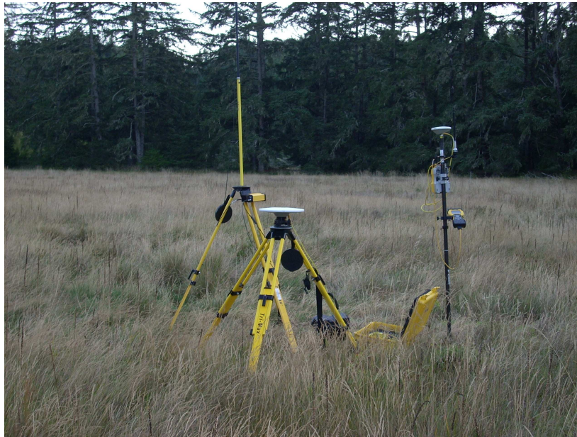
Figure 14 - DGPS Base Station, Radio Link, and GPS rover used for data collection in the South Slough.
