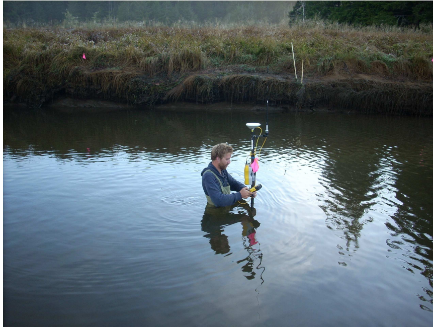
Figure 16 – Wading Winchester Creek with the GPS Rover (RTK pole). Lower tides were required to wade some sections of the study area.
