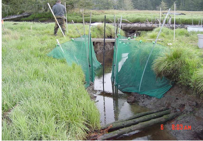
Figure 8. Photo showing fyke net and camera set up at mouth of Dalton Creek.
