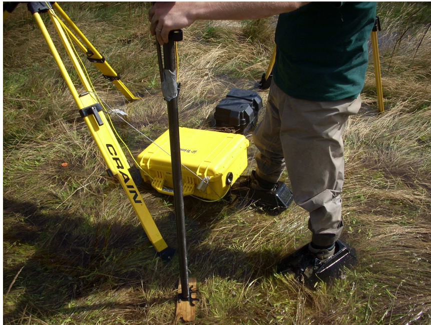
Figure 15 – The foot of the 2-meter RTK pole was modified with a flat base to prevent the tip from sinking into the channel mud.
