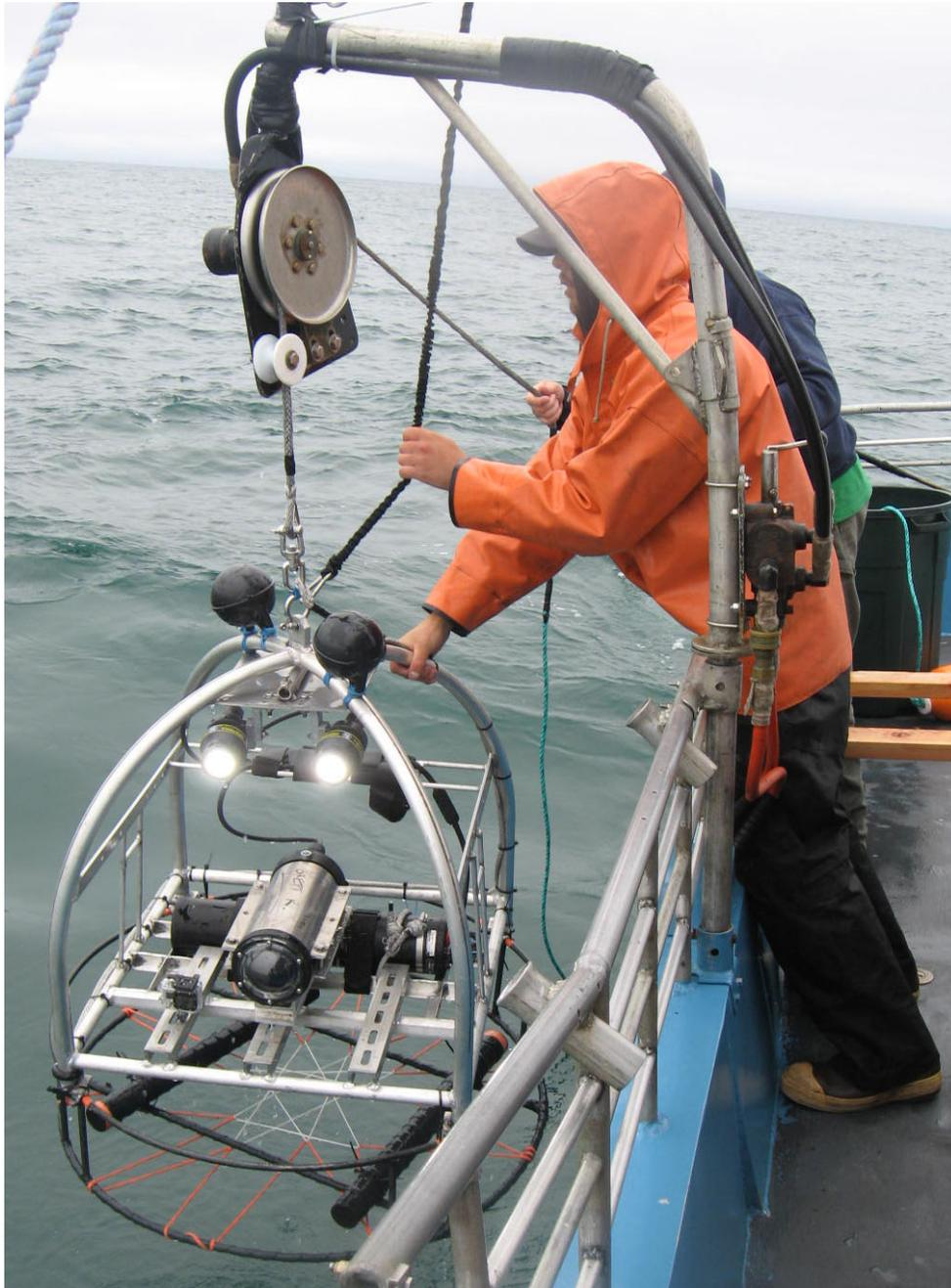
Figure 1. Video lander. The aluminum lander frame that protects the camera housing, battery housing, and lights is mounted on a weighted sacrificial base. The video lander was dropped over the side of the vessel and allowed to sink freely to the bottom with a line and floating buoy attached for retrieval. The lander was retrieved with a hydraulic winch then lifted over the side of the vessel by attaching a line from an electric winch.
