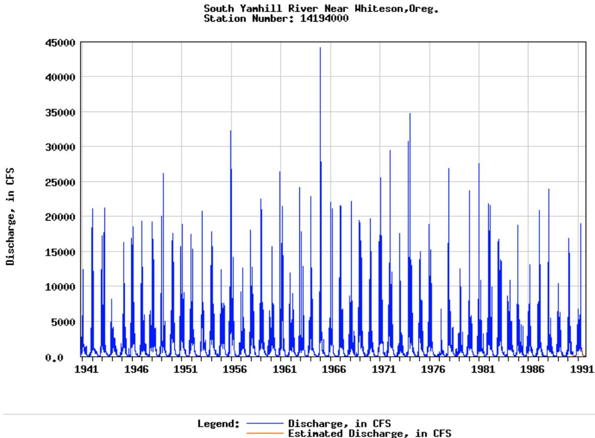
Flow data was collected on the south Yamhill River at Whiteson gaging station (gage # 1419400) located just off Hwy 99 north of Whiteson where the river flows under the road. It drains an area of 502 sq. miles, and is located 82.3 feet above sea level (Water Resources website).
